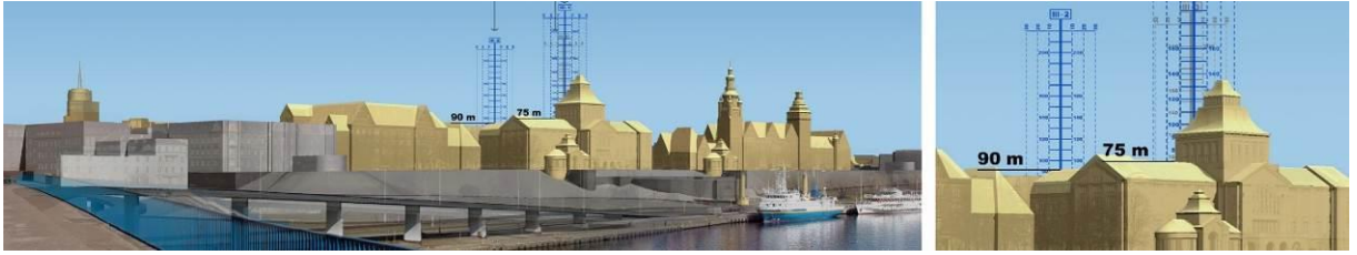
Simulations of Szczecin's (Poland) panoramas with height rulers placed in locations of planned tall buildings. The method helped determining numbers and limit heights above which specific buildings can be seen above skyline
